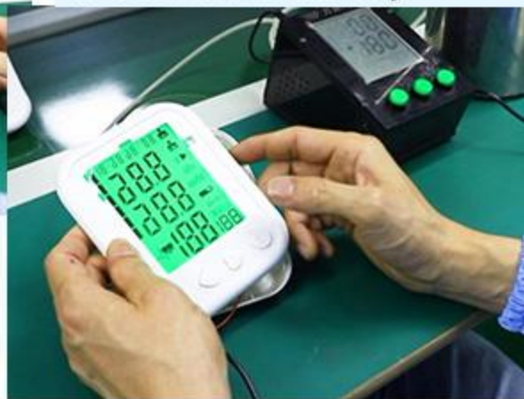
Blood pressure monitor simulation detection this is the most importance step to ensure the accuracy
